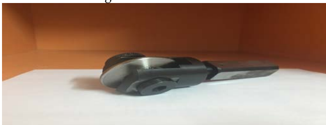
Figure 2- Roller Burnishing Tool
