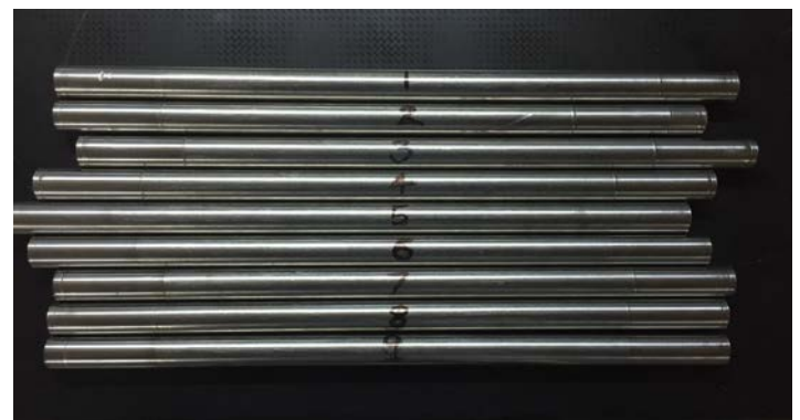
Figure 3- Titanium Grade-5 Specimen Rod
